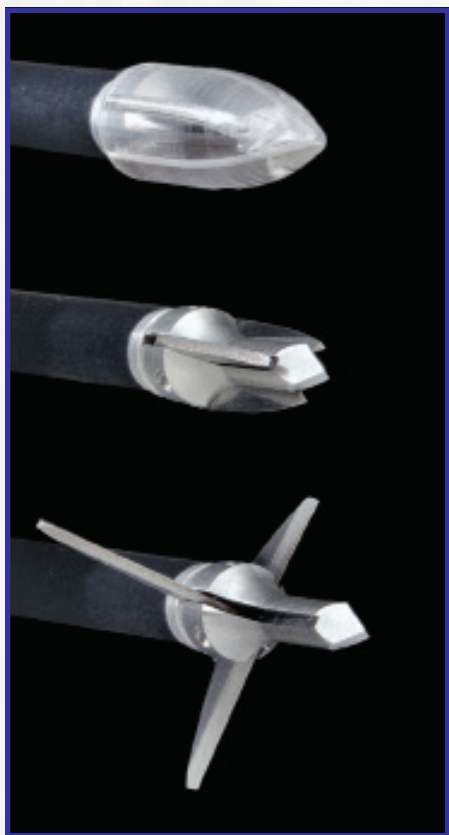
Sullivan Industries designed the Shape Shifter to deliver true field point accuracy at the highest arrow speeds by enclosing the mechanical head in an Exo-Cover designed to break away on impact as it helps to ramp the blades open. The head is all-stainless-steel, weighs 100 grains and cuts a 1-1/4 inch circle. The blades are a sturdy .040 of an inch thick.
