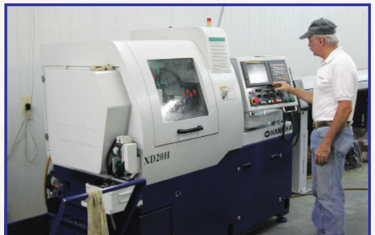
Dennis Sullivan makes adjustments on one of the modern CNC machines. A 12 foot automatic bar-loader, which allows this machine to run for hours unattended, is visible in the background.
